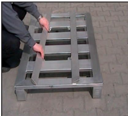
To take off or to move the wedges please fold up the wedges (remove them)- now the wedges are flexible for a new width or removable
