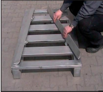
Insert safetywedge diagonal into the pallet deck
